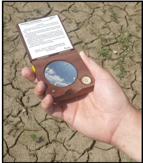
Figure 2. A spherical densiometer was used to estimate canopy cover above each wetland.
